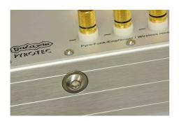
All devices that have been manufactured later than June 2010 are equipped with a screw on the right long side of the housing. A tube which has been filled with drying agent has been installed in the device behind that screw. Due to that, the user is enabled to easily change the drying agent by himself. All other equipment with desiccant has always been equipped with a screw for replacing the desiccant.
